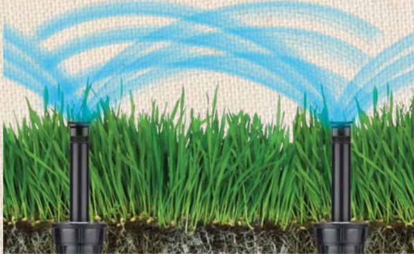
2. **Fill in the trenches** once the sprinklers have been installed. **Bury the sprinkler heads** so the tops are about 1/4 inch above the soil. Make sure to properly pack the trenches to avoid collapse during watering.
